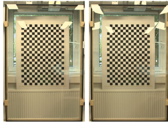
1. HDR images of IGUs with different levels of deformation for comparison of optical behaviour
