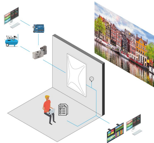
2. Proposed experiment setup with air pressure system for glass deformation
