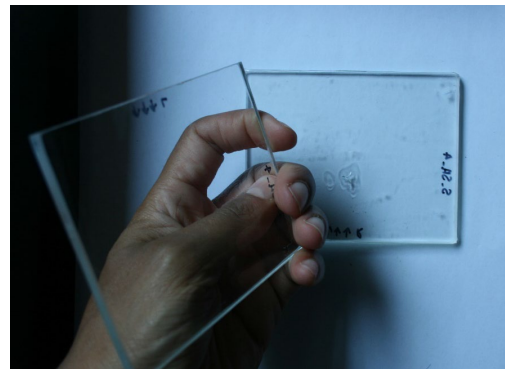
Separated PVB-laminated glass
